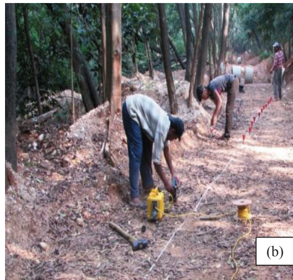
Fig. 4: (a) Field data acquisition using 25 MHz RTA on the site and (b) Typical field set for MASW survey
