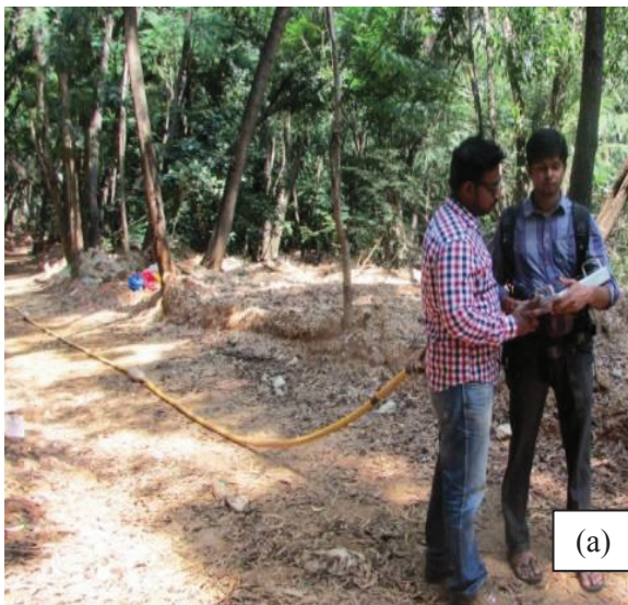
Fig. 4: (a) Field data acquisition using 25 MHz RTA on the site and (b) Typical field set for MASW survey
